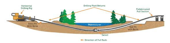
The river and watercourse crossing construction technique may be refined during the detailed engineering and design phase.
