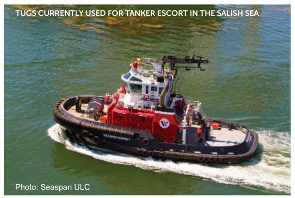
Seaspan Osprey (81-mt Bollard Pull) - Operated by Seaspan Marine
