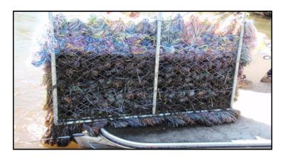
catch non-floating oil. They can consist of pom-pom type materials that are strung together and submerged. Sorbents are used for both detection and recovery.
