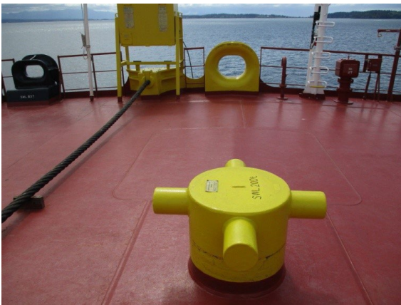
Figure 7: Examples of vessel's towing strong points that are suitable for escort tug line securing.
